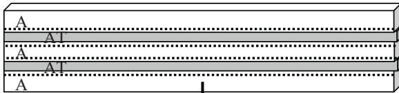
Fig. 1. Schematic illustration of the designed laminated structure with five layers showing a bend bar and the notch orientation with respect to the layers. 14 The thick external and central alumina layers (A) are represented with white colour and have a thickness of \cong 1800 \mu\text{m} . The thin alumina + 10 vol.% aluminium titanate internal composite layers (AT) are represented with grey colour and have a thickness of \cong 300 \mu\text{m} . Dashed lines indicate the position of large grained alumina interfaces due to titania diffusion.
